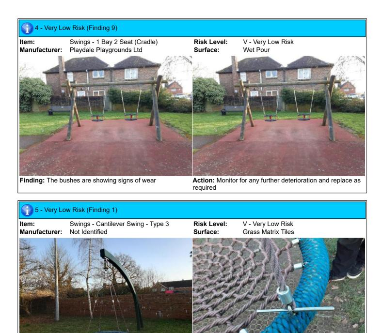
**Finding:** The connecting links are in excess of 8.6mm and less than 12mm and fail the requirements of BS EN 1176 Part 1; clause 4.2.13, Chains
