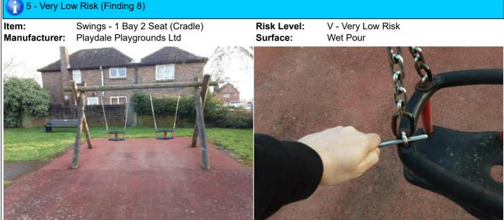
**Finding:** The connecting links are in excess of 8.6mm and less than 12mm and fail the requirements of BS EN 1176 Part 1; clause 4.2.13, Chains
