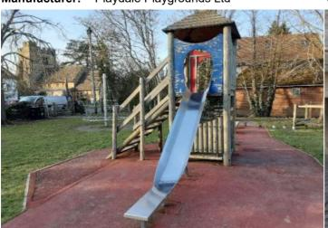
Finding: The item fails to meet the requirements of BS EN Action: Monitor - No remedial work recommended 1176 Part 1 4.2.7.2 head and neck entrapment in the barriers and/or steps
