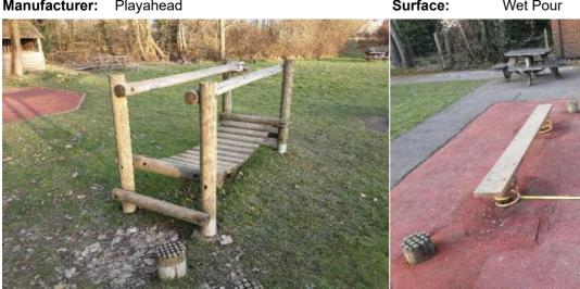
Finding: The surfacing dimensions are short and do not meet with the requirements of the current applicable standard
